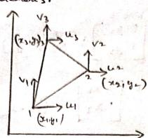
consider a typical CST clouds with nodes 1,2 and 1 as shown in Fig. let the nodel displacements be u, u2 4, V, V2 and Vs
